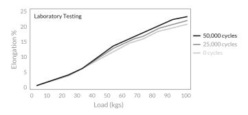
The above graph shows that even after repeated stretching over 50,000 cycles at 100kgs, the Black Cat® product maintains it's resilience without collapse. This random testing also checks to ensure no variation more than +5% / - 5% occurs.
